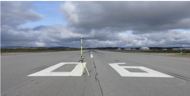
Figure 2: Ground Control Point (GCP) collection on the Airport
